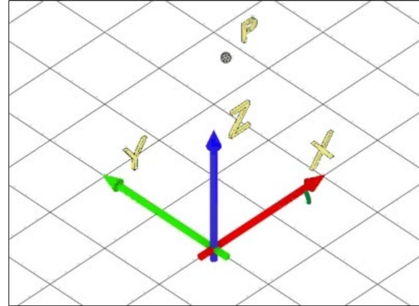
$$\begin{array}{c} x \\ |y| \\ z \end{array} = R \cdot \begin{array}{c} X \\ Y \\ Z \end{array} \quad R = R_{\kappa} \cdot R_{\phi} \cdot R_{\omega}$$
